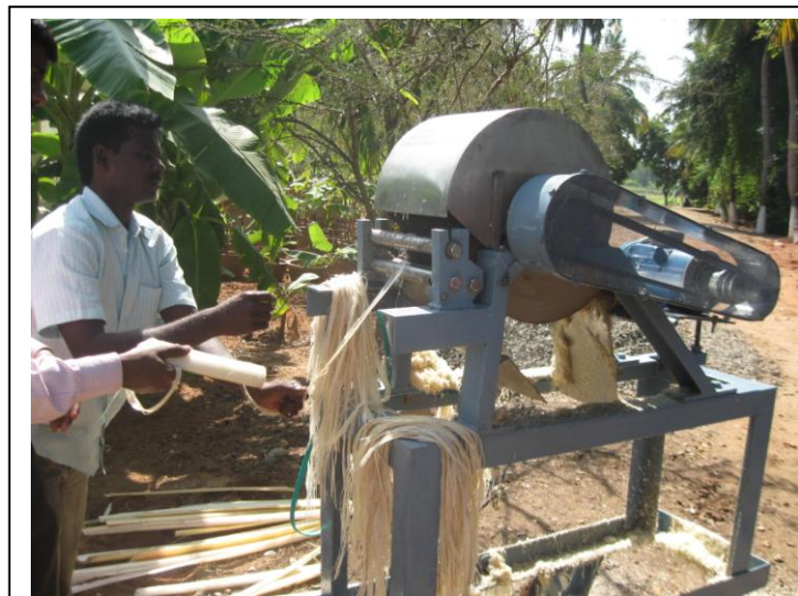
Machine extraction of fibre from banana stem
